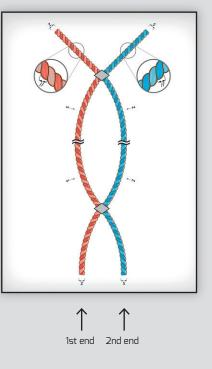
Multi-purpose twisting system for carpet BCF yarns; each module produces 2 ends of 2 ply or 2 ends of 3 ply yarn in 1 single step. High speed twisting with maximum bulk and no singles twist.
