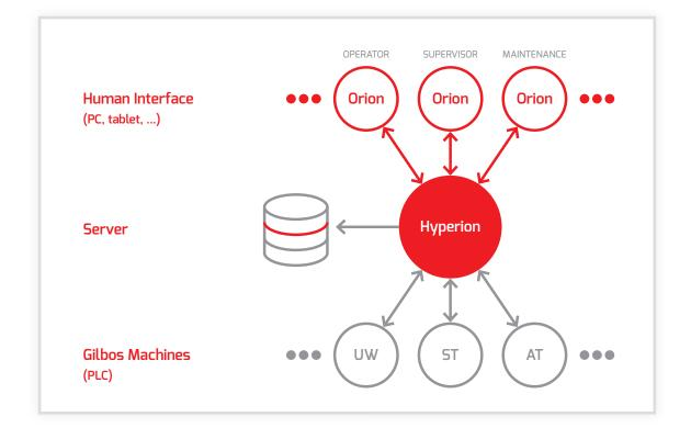
The Gilbos Hyperion control system controls all the vital entanglement parameters such as speed, air pressure and yarn tension.
