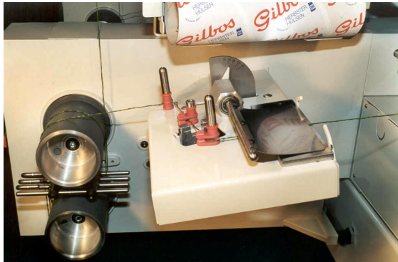
Random or (Step)Precision winding
