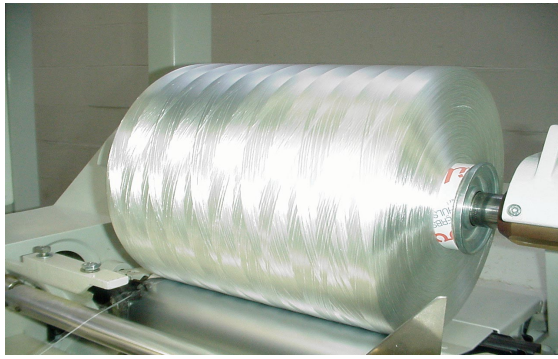
Yarn guiding by swivelling arm
