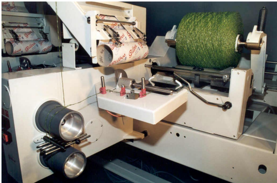
Yarn guiding by swivelling arm
