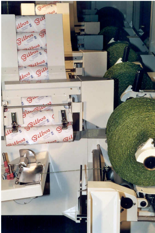
Extended tube magazines up to 8 tubes
