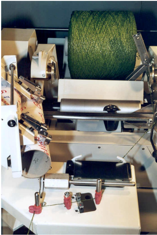
Extended tube magazines up to 8 tubes
